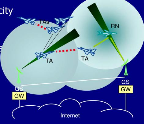
TA – test article GS – ground station RN – relay node GW – gateway
