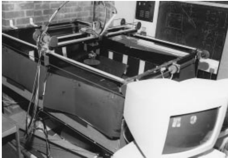
FIG. 3. The Gantry viewed from above. The horizontal girder moves along the side rails, and the robot is suspended from a platform which moves along this girder.
